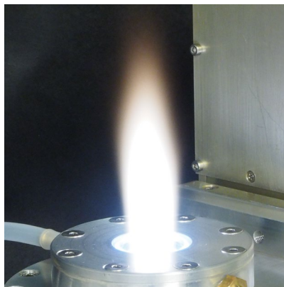
Microwave plasma at atmospheric pressure: In a resonator system, microwaves ignite the gas flowing in and form a plasma, which is then blown into a reactor. (© IGVP, Universität Stuttgart)
