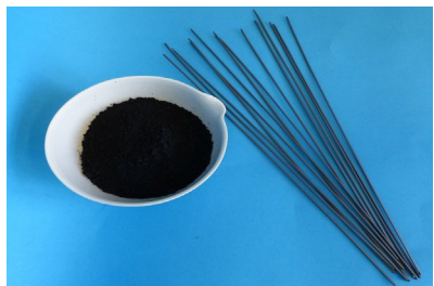
A green body hollow fiber is spun from the ceramic powder using a binder and then sintered. The perovskite capillaries shown here have a diameter of 2 mm and a wall thickness of 150 µm. (© Fraunhofer IGB)
